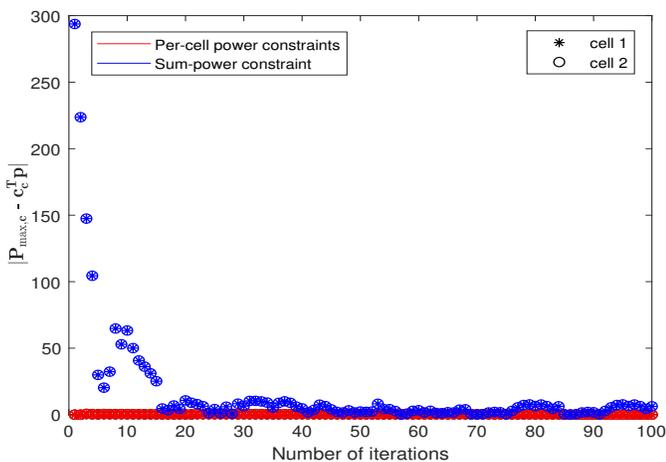
Fig. 2: Difference between the per cell total power and its respective power constraint VS number of iterations: SNR = 30 dB,  $C = 2$ ,  $K_c = 3$ ,  $M_c = 20$ ,  $N_k = d_k = 2$ ,  $P_{\max,1} = P_{\max,2}$ .
