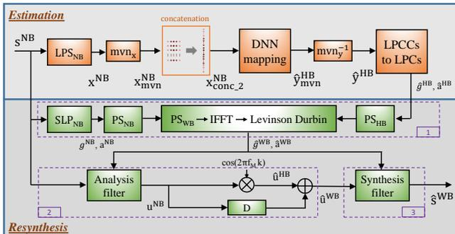
**Fig. 1.** A block diagram of the baseline ABE system. Diagram adapted from [23].
