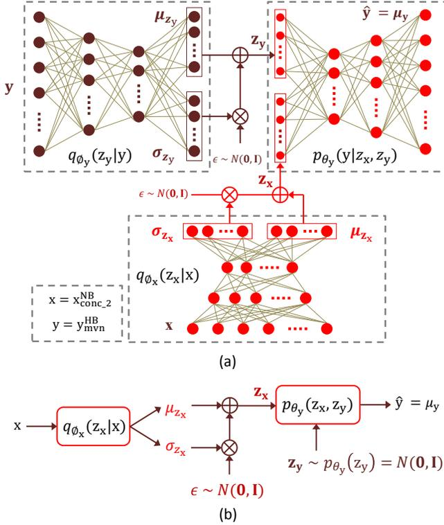
**Fig. 2.** (a) The proposed CVAE-DNN scheme during training (or reconstruction) phase and (b) testing (or prediction) phase.
