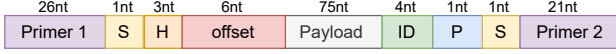
Figure 2 – Format of the oligos - S denotes the sense nucleotide which determines whether a strand is reverse complemented when sequenced. P is a parity check nucleotide while the ID is an identifier of the image so to be distinguished from other data that may be stored. H is a specific header, Offset specifies the chunk’s data position in the encoded sequence and Payload contains the encoded chunks.
