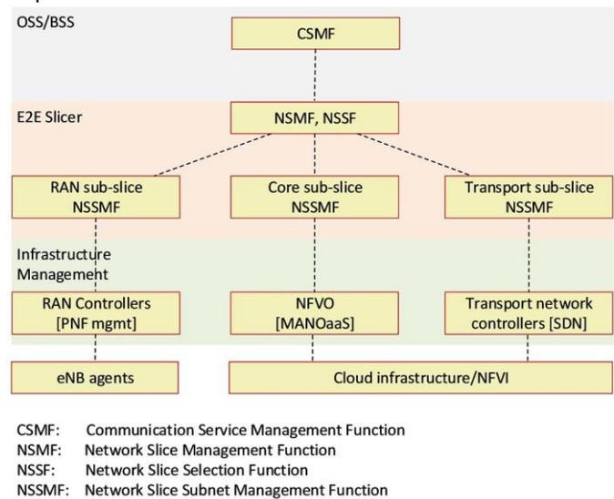
Fig. 1: High-level view of our E2E network slicing architecture. Our design features an E2E Slicer which implements NSMF and NSSF components. It supports the integration of PNFs for RAN slicing and different MANO stacks per slice type and interacts with them via different NSSMF components per sub-slice.
