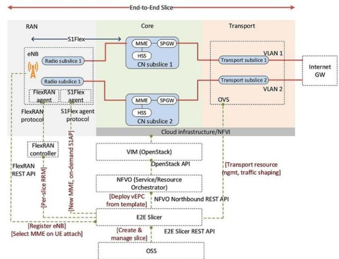
Fig. 3: Detailed architecture of the proposed framework.
