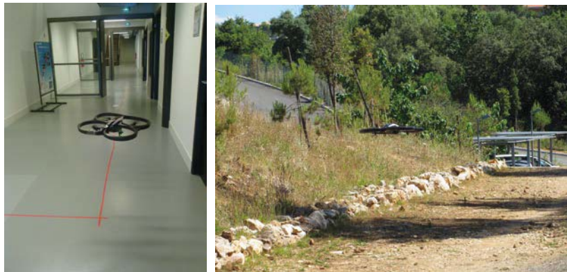
Figure 1: Left picture: a drone can follow a line on the floor with no human control (indoor navigation). Right picture: the drone must also be able to navigate autonomously outdoor.
