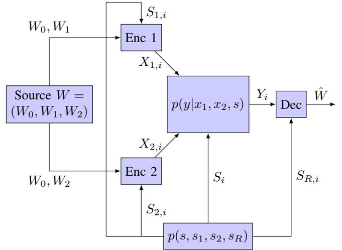
Fig. 1. State-dependent multiple-access channel with common message  $W_0$ , independent messages  $W_1, W_2$ , D-CSIT  $S_1, S_2$  and imperfect CSIR  $S_R$ .
