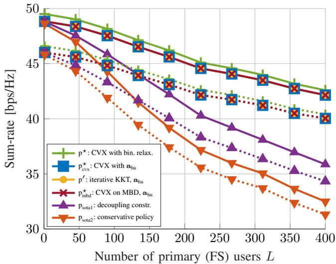
Fig. 4. Sum-rate vs.  $L$  for  $P_{\text{max}} = 47\text{dBm}$ .
