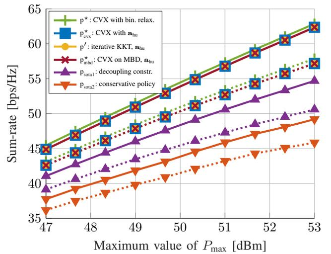
Fig. 5. Sum-rate vs.  $P_{\text{max}}$  for  $L = 200$ .
