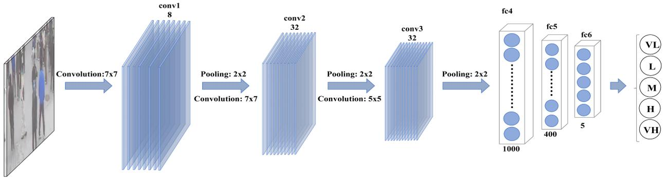
Fig. 1. The proposed crowd CNN architecture composed of three convolutional layers and three fully connected layers for crowd level classification: 5 classes of density: Very Low (VL), Low (L), Medium(M), High(H), and Very High(VH)
