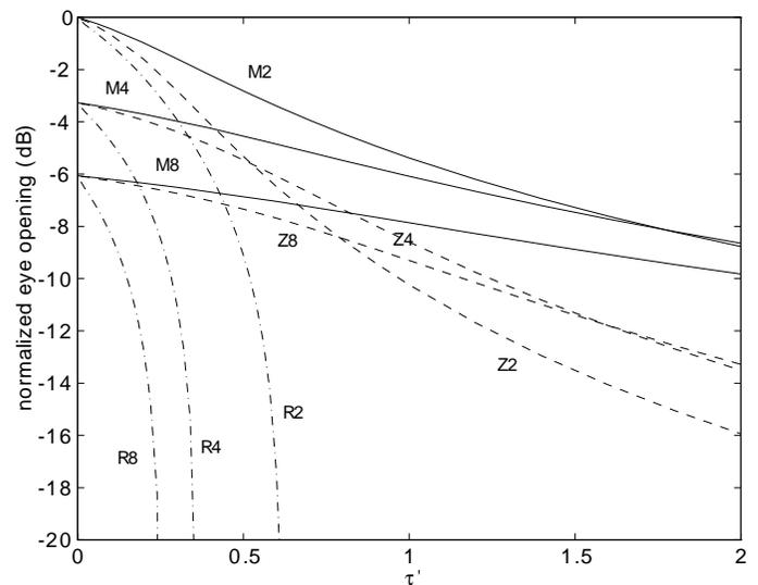
Figure 2: The optical filter is a Fabry-Perot interferometer. The curves are labelled as follows: (M) matched filter curve, (Z) zero-forcing filter, (R) rectangular filter, and (2,4,8) level signaling.
