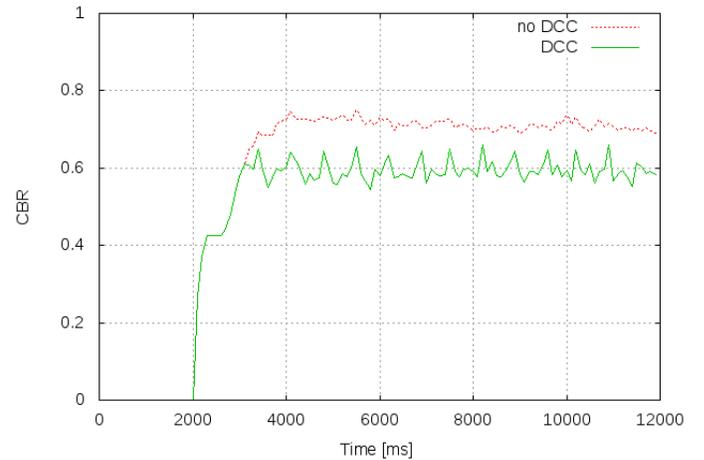
Fig. 11: CBR vs time for 250 vehicles in slow highway scenario
