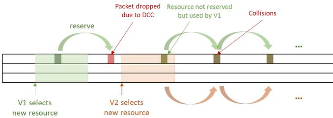
Fig. 15: Collisions due to packet drop (DCC mechanism)
