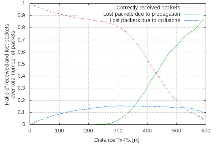
Fig. 10: Ratio of received and lost packets over number of sent packets for 200 vehicles in slow highway scenario
