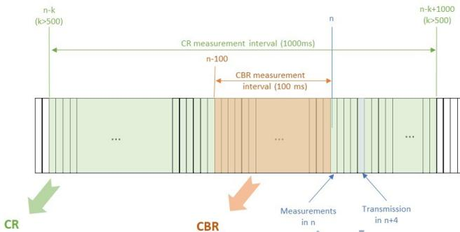
Fig. 6: CBR and CR calculations in DCC mechanisms
