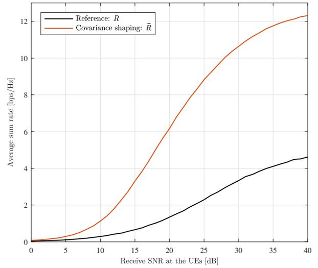
Figure 4. Average sum rate versus receive SNR at the UEs with the same uplink pilot sequence for the reference and covariance shaping scenarios.
