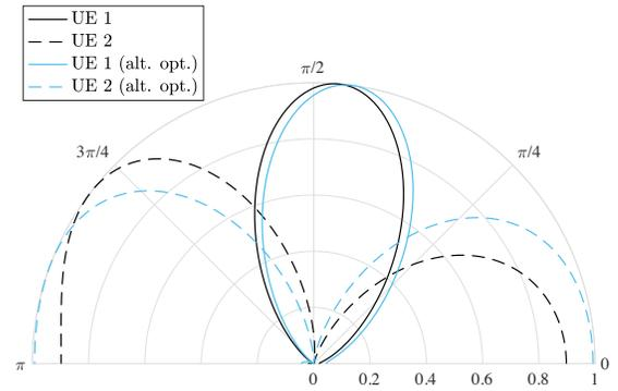
Figure 2. Antenna diagram of the covariance shaping vectors at the UE-side obtained solving (14) and (15) (alternate optimization).
