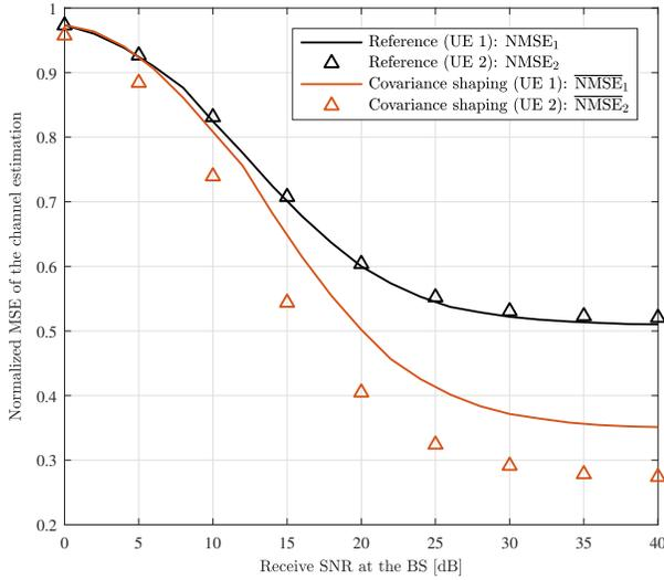
Figure 3. Normalized MSE of the channel estimation versus receive SNR at the BS with the same uplink pilot sequences for the reference and covariance shaping scenarios.
