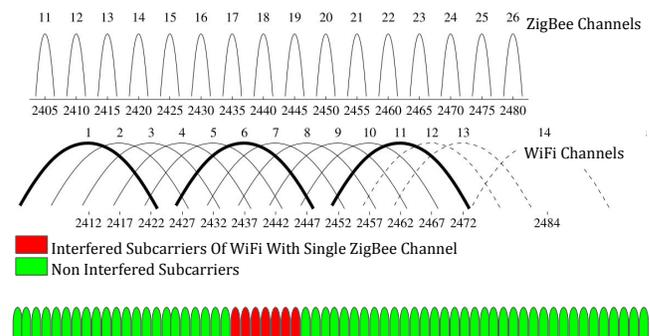
**Fig. 1. WiFi Subcarriers and Single ZigBee Channel Overlap**
