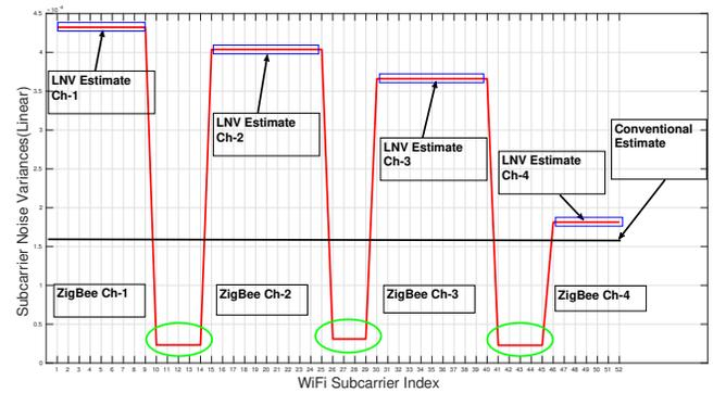
Fig. 3. Conventional vs LNV Estimates: Single WiFi Channel Interfered by 4 ZigBee Channels
