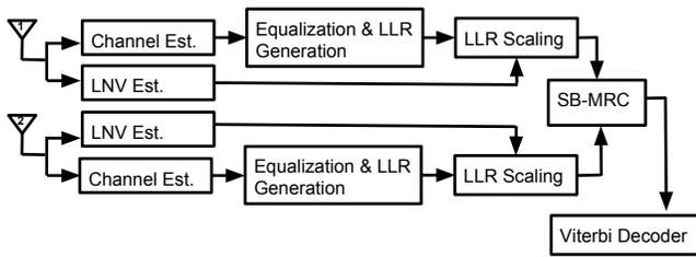
Fig. 4. Schematic of Section 2.2: Dual Antenna Solution
