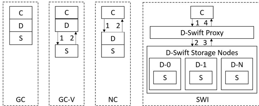
Fig. 5.1 *Compute-to-Data path* for different scenarios during read operations.
