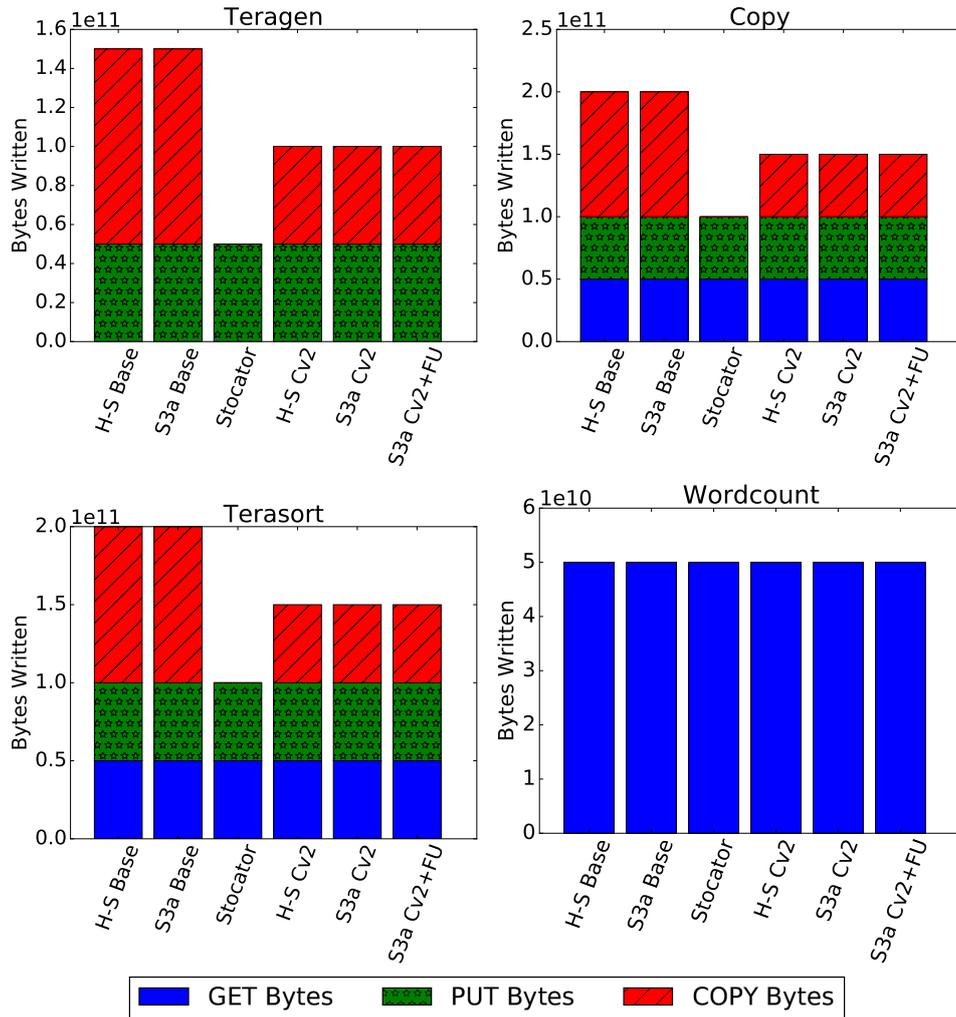
Fig. 6.5 Object Storage bytes read/written comparison
