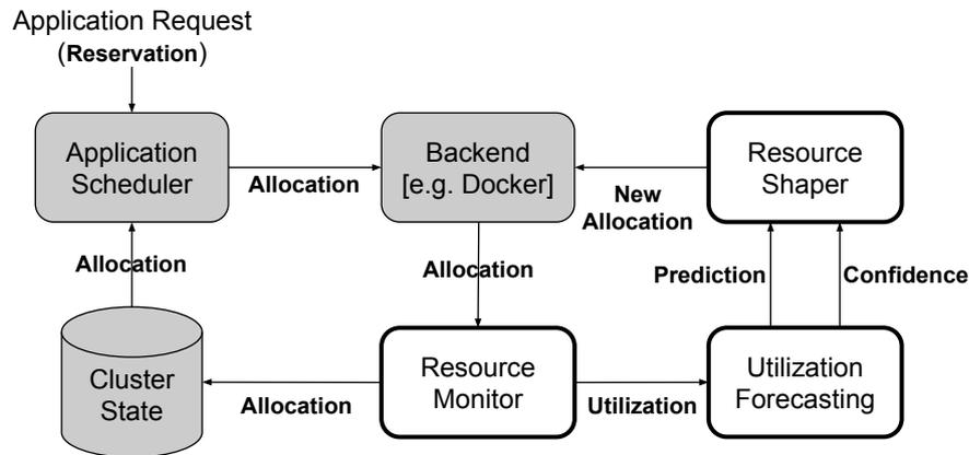
Fig. 4.1 System overview: shaded boxes represent existing components, white boxes indicate new components presented in this work.
