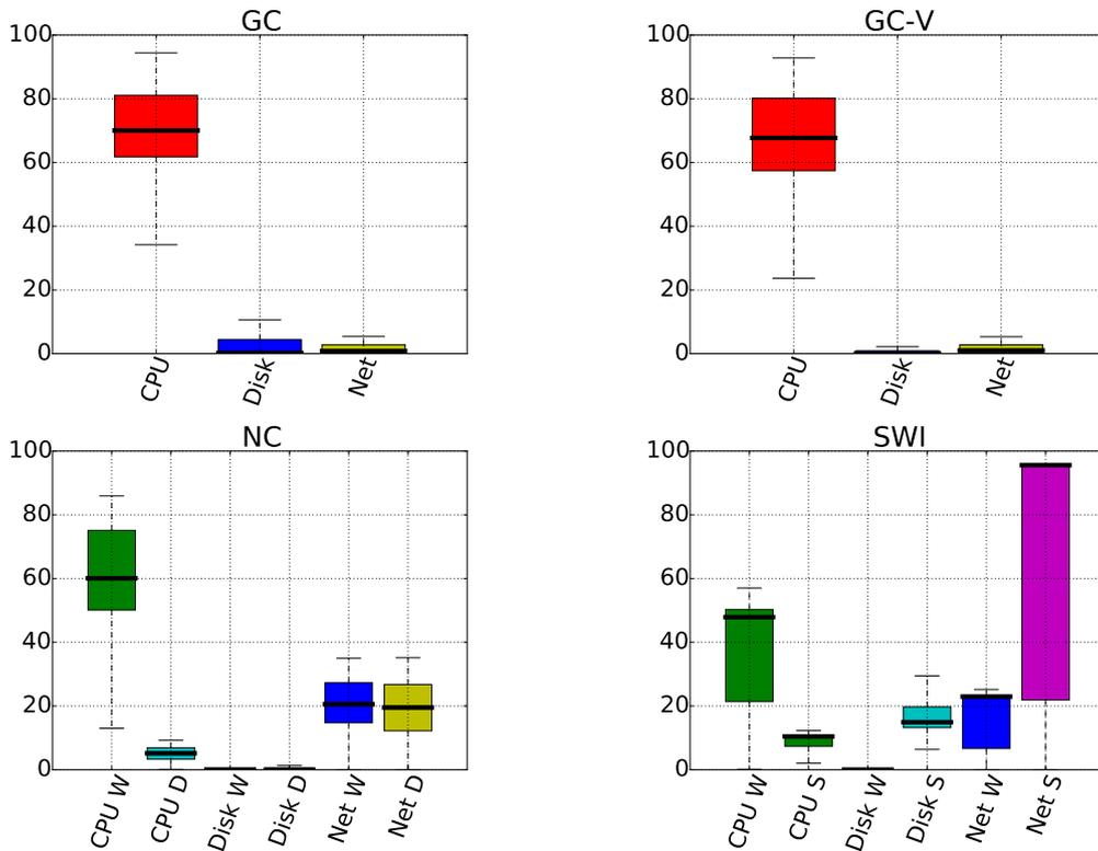
Fig. 5.3 Resource utilization with the TPC-DS workload in different scenarios. The ticks on the X axis “W”, “D” and “S” stand, respectively for worker, datanode and Swift machines. The resource utilization reported is a global average across all instances of each layer. The network utilization between the GC-V and GC scenarios is similar because volumes’ network is opaque to the Operating System and, therefore, counted in the disk utilization.
