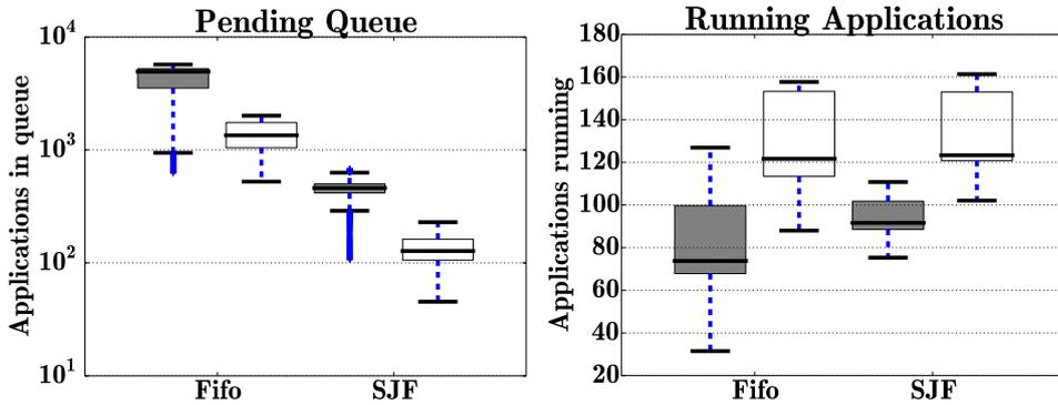
Fig. 3.4 Comparison of queues size for FIFO and SJF between our flexible scheduler and the baseline. The white boxes (right box of every group) correspond to our flexible algorithm, gray boxes to the baseline.
