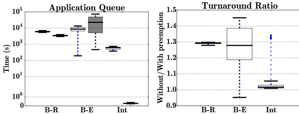
Fig. 3.9 On the left, comparison of queuing time distributions between scheduling with and without preemption. White boxes (left box of every pair) correspond to a *non-preemptive* system, gray boxes to our preemptive algorithm. On the right, turnaround ratio distributions between scheduling with and without preemption. *B-E* stands for batch elastic applications, *B-R* stands for batch rigid applications and *Int* is for interactive applications.
