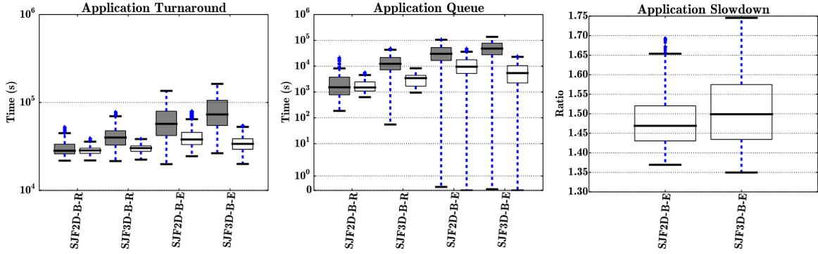
Fig. 3.6 Comparison of turnaround and queue time distributions, and application slowdown distributions for the SJF policy with different definitions of size. White boxes (right box of every pair) corresponds to our flexible scheduler, gray boxes correspond to the baseline. *B-E* stands for batch elastic and *B-R* stands for batch rigid applications.
