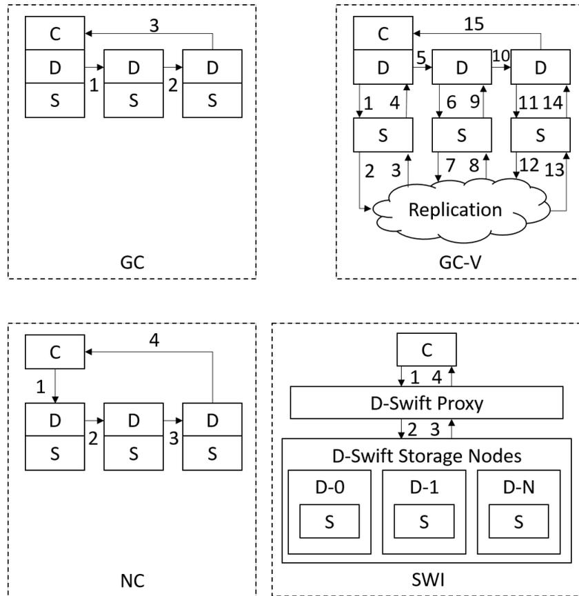
Fig. 5.2 *Compute-to-Data path* for different scenarios during write operations.
