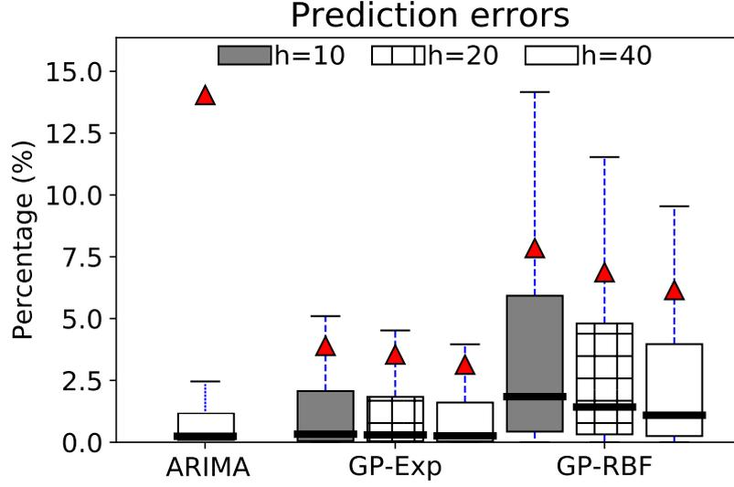
Fig. 4.2 Boxplot showing error distribution of predicted utilization for a collection of time series in our academic cluster with different history points and, in case of GP, different kernels. The red triangle is the mean.
