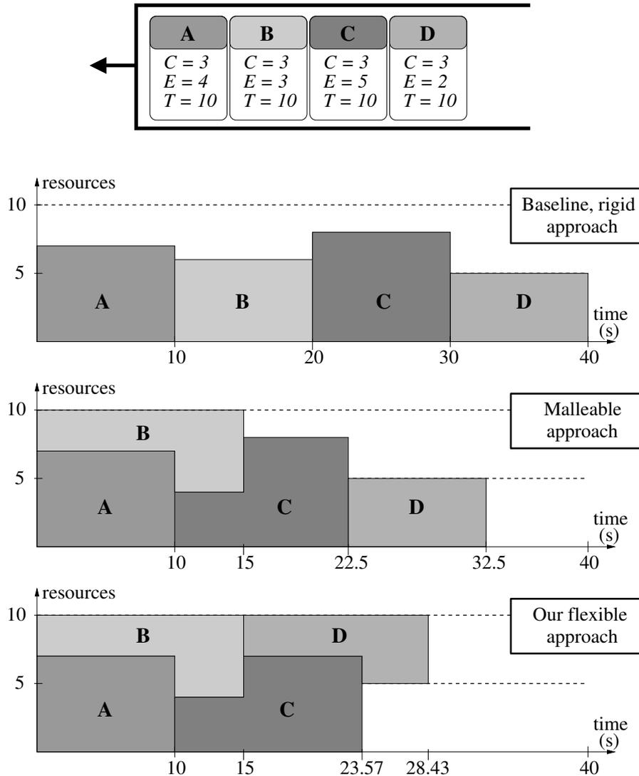
Fig. 3.1 Illustrative examples of request scheduling: (top) rigid, (middle) malleable, (bottom) flexible approaches.
