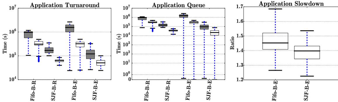
Fig. 3.3 Comparison of turnaround and queue time distributions, and application slowdown distributions for FIFO and SJF policies. White boxes (right box of every pair) corresponds to our flexible scheduler, gray boxes correspond to the baseline. *B-E* stands for batch elastic and *B-R* stands for batch rigid applications.
