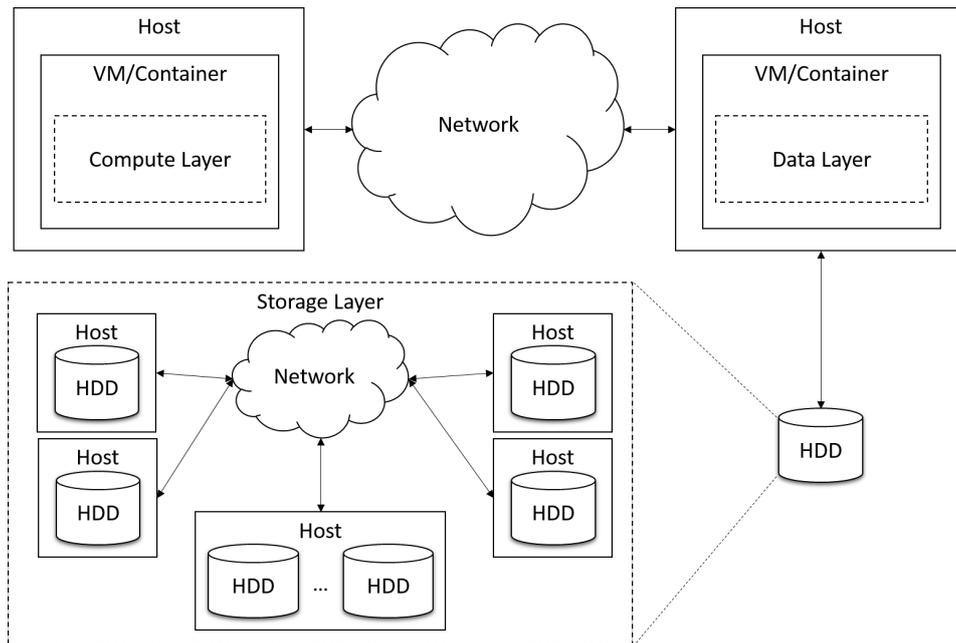
Fig. 2.2 Logical components in an analytics cluster.
