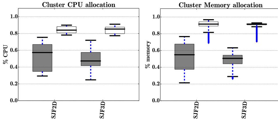
Fig. 3.8 Comparison of resource allocation distributions for the SJF policy with different definitions of size. White boxes (right box of every pair) corresponds to our flexible scheduler, gray boxes correspond to the baseline.
