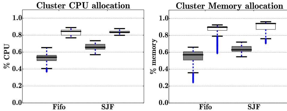
Fig. 3.5 Comparison of resource allocation distributions for FIFO and SJF policies, between our flexible scheduler and the baseline. White boxes (right box of every pair) correspond to our approach, dashed boxes to the baseline.
