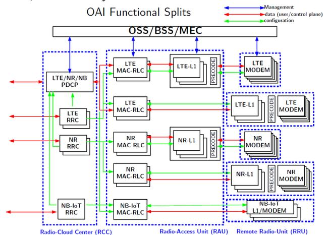
Fig. 2. Software architecture of openairinterface5g
