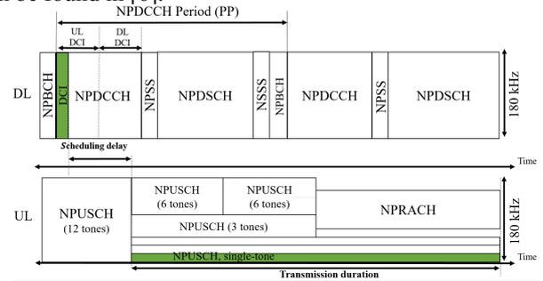
Fig. 3 Timing diagram of NB-IoT physical channels.
