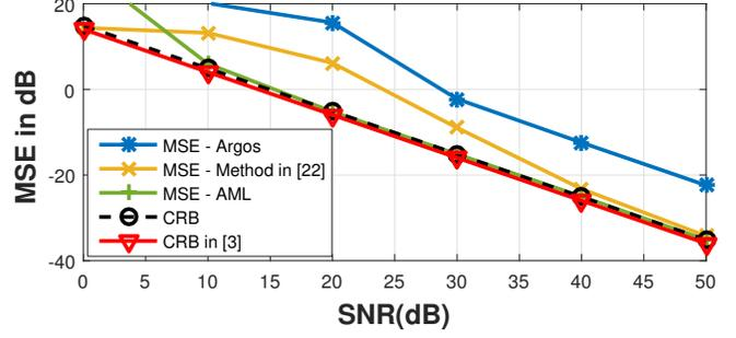
**Fig. 2.** Comparison of single antenna transmit schemes with the CRB ( $G = M = 16$ ).
