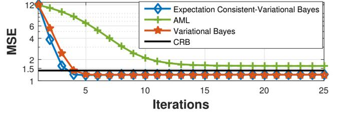
**Fig. 3.** Convergence of the various iterative schemes for  $M = 16$  and  $G = M$ .
