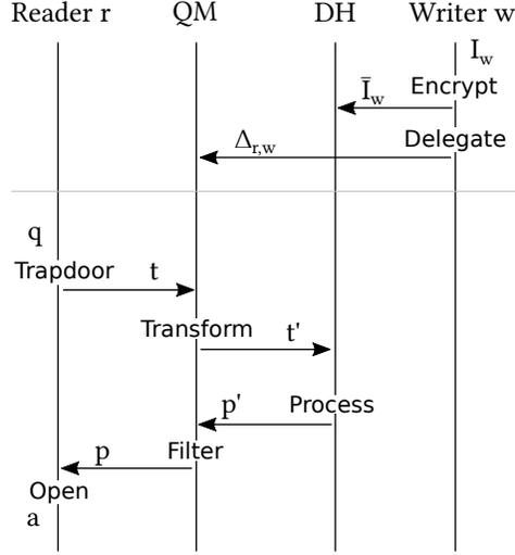
Figure 2: Illustration of the protocol flow showing encryption, delegation and search
