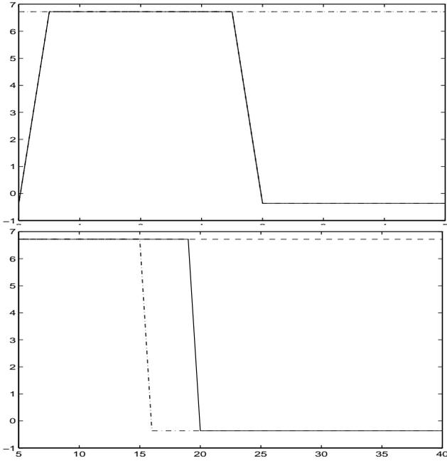
Figure 2: SINRM<sub>1</sub> at the output of **C1**, **J2** and **C2** as a function of  $c_v$ , ULA,  $N = 4$ ,  $P = 2$ ,  $\theta_1 = 0$ ,  $\theta_2 = 10$  degrees, SNR = 5 dB,  $c = -0.1$ : top,  $c = -1$ : bottom
