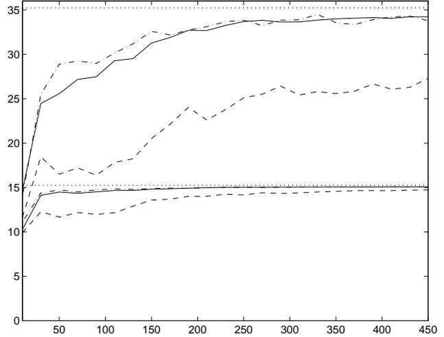
Figure 3: SINRM<sub>1</sub> at the output of **C1**, **J2** and **C2** as a function of  $K$ , with ULA  $N = 4$ ,  $P = 2$ ,  $\theta_1 = 0$ ,  $\theta_2 = 20$  degrees, SNR = 10, 30 dB,  $c_1 = -1$ ,  $c_2 = 0$
