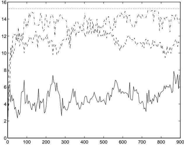
Figure 4:  $\text{SINRM}_1$  at the output of **C1**, **J2** and **C2** as a function of  $K$ , with ULA,  $N = 4$ ,  $P = 2$ ,  $\hat{P} = 2$  or  $3$ ,  $\theta_1 = 0$ ,  $\theta_2 = 20$  degrees,  $\text{SNR} = 10$  dB,  $c_1 = c_2 = -1$ .
