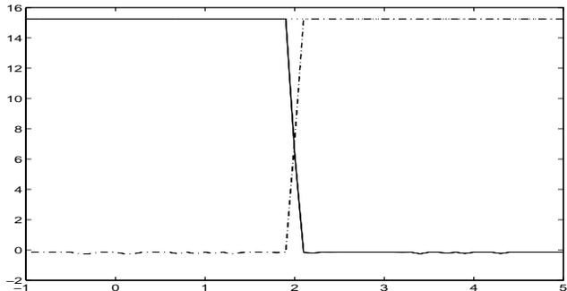
Figure 1:  $\text{SINRM}_1$  as a function of  $c_2$ , with  $P = 2$ ,  $N = 4$ , ULA,  $\theta_1 = 0$ ,  $\theta_2 = 20$  degrees, SNR = 10 dB,  $c_1 = -2$ ,  $\mu = -1$ : solid,  $\mu = +1$ : dashdotted
