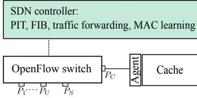
Fig. 5. Architecture of a stateless S/N-DN node.
