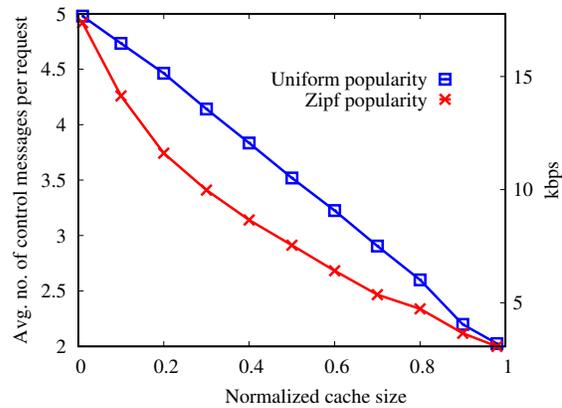
Fig. 13. Control traffic for the stateless approach, for  $d_{ss}=100$  ms,  $d_{sc}=100$  ms and one request per second.
