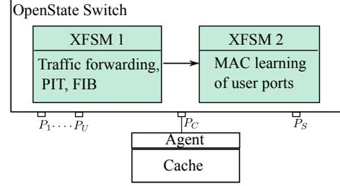
Fig. 4. Architecture of a stateful S/N-DN node.
