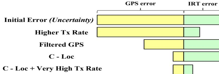
Figure 2: Conceptual Representation of Awareness Error due to GPS and IRT.
