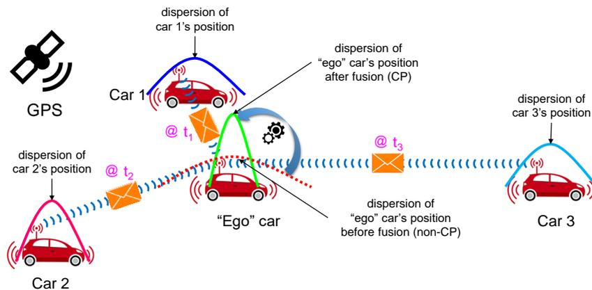
Figure 1: “Ego” car receiving asynchronous CAMs from one-hop “virtual anchors” to perform distributed CLoc. The dispersion of CLoc location estimates (through both GNSS and ITS-G5) is expected to be lower than that of non-CLoc estimates (i.e. standalone GPS)
