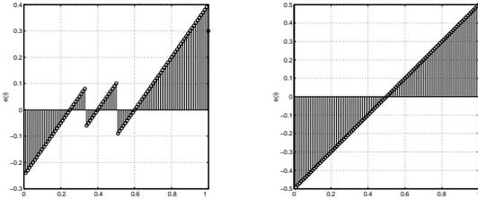
Figure 3: 4-PAM: The stationary points on the line  $s_1 = s_2$  for DD and Sato, respectively
