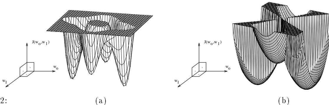
Figure 2: (a) CMA and NSWCMA ( $M=1$ ) cost functions in a case of two equalizer parameters
