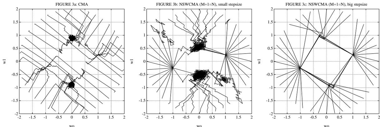
Figure 3: A comparison of CMA and NSWCMA ( $M=1$ ) for an AR(1) channel
