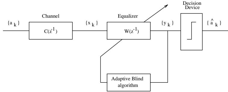
Figure 1: A typical blind equalization scheme
