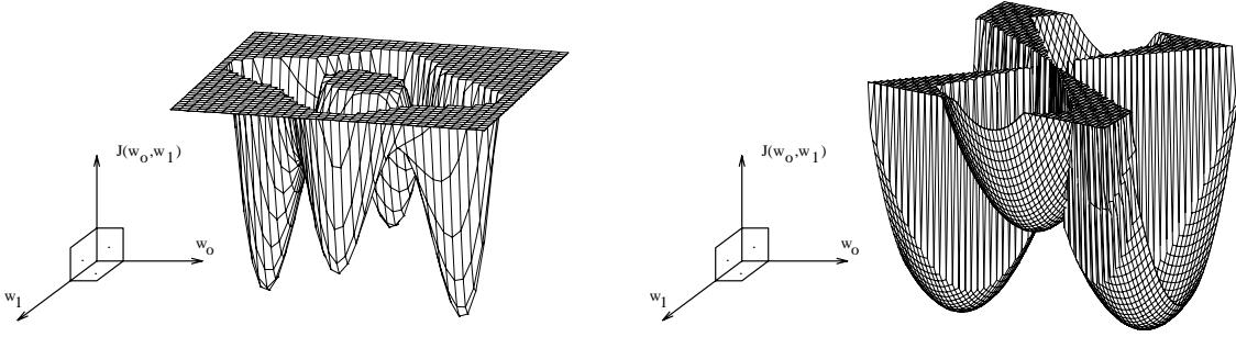
Figure 2: (a) CMA and NSWCMA ( $M=1$ ) cost functions in a case of two equalizer parameters
