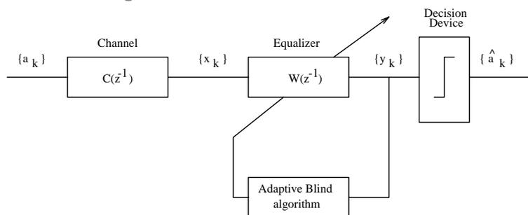
Figure 1: A typical blind equalization scheme
