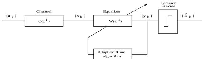
Figure 1: A typical blind equalization scheme
