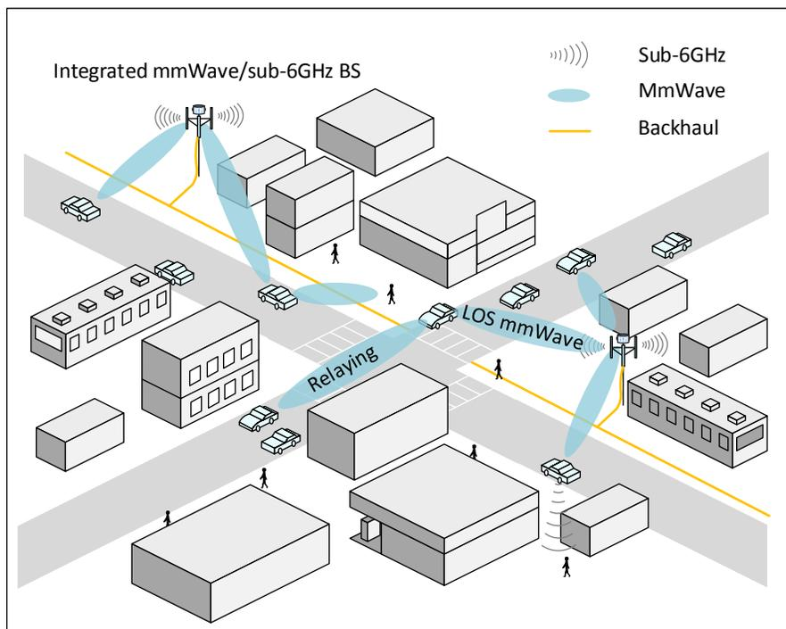
**Figure 1.** Relaying in the integrated mmWave/sub-6GHz 5G network.
