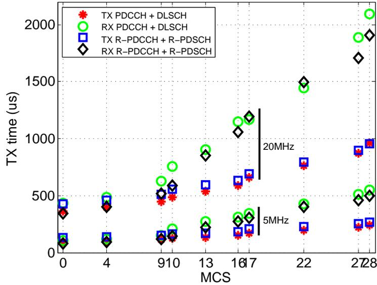
Figure 6: Total TX and RX processing time for PDCCH/PDSCH and R-PDCCH/R-PDSCH
