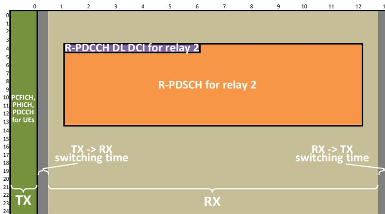
Figure 3: Example of SF allocation for Relay DL channel shared between access and backhaul in a MBSFN SF at the relay
