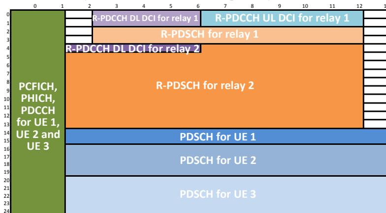
Figure 2: Example of SF allocation from DeNB DL channel
