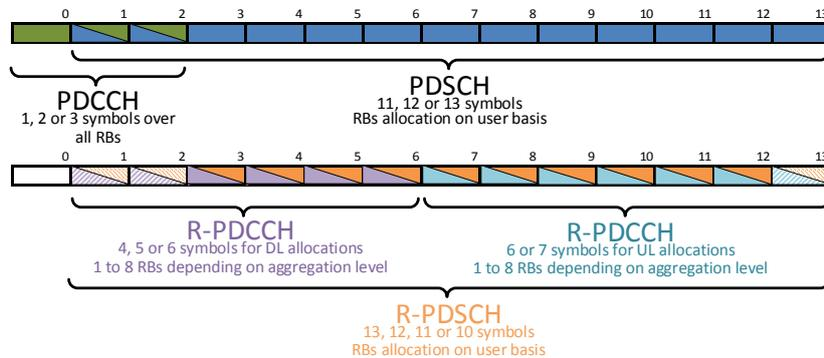
Figure 1: SF flexibility for UE DL channels ( $Uu$ ) (top) - relay DL channels ( $Un$ ) (bottom)
