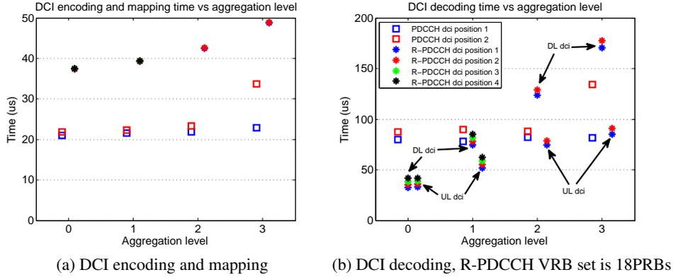
Figure 5: R-PDCCH and PDCCH computational time for 10MHz channel
