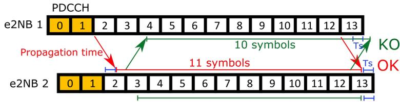
Figure 4: Transmission problem for non subframe synchronized e2NBs
