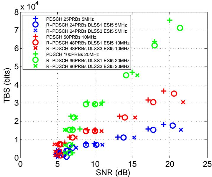
Figure 7: Minimum SNR to decode 75% of the transmission for different channel bandwidth, DL.StartSymbol (DLSS) and second slot End Symbol Index (ESI). Maximum PRB allocation for one user. Different TBS values are obtained from different MCS values (0,4,9,10,16,17,22,27,28).
