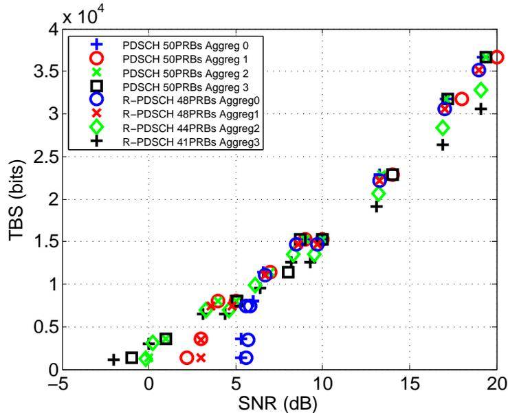
Figure 8: Minimum SNR to decode 75% of transmissions for different aggregation level. 10MHz channel with maximum PRB allocation for one user. Different TBS values are obtained from different MCS values (0,4,9,10,16,17,22,27,28).
