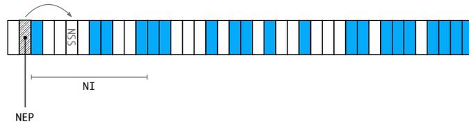
Figure 3: **STDMA**: network entry phase: choice of the **NEP** slot and of the **NSS**
