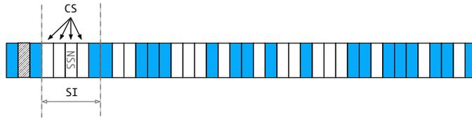
Figure 4: **STDMA**, network entry phase: **SI** and **CS** compilation.
