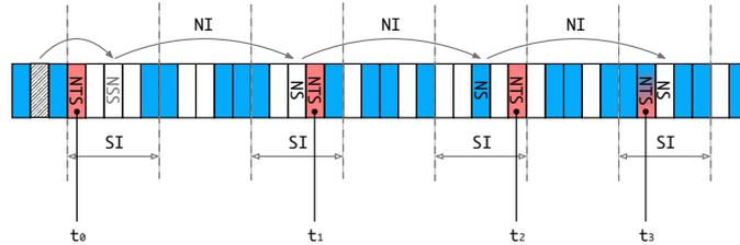
Figure 6: **STDMA**, network entry phase: **NTS** selection and **NEP** transmission
