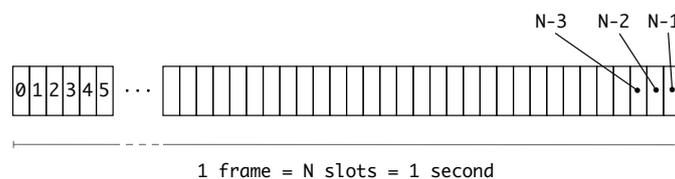
Figure 1: [STDMA](#): channel organization into slots and frames
