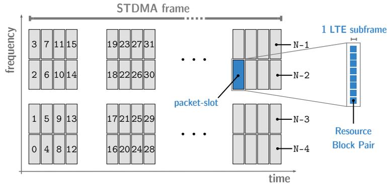
Figure 8: Construction of slotted system over the LTE SL. It is worth mentioning that “STDMA frame” and the “LTE subframe” are unrelated entities: the former is the basic period of the STDMA protocol, whereas the latter refers to the set of RBs contained in the whole bandwidth in one TTI
