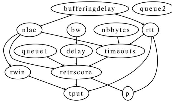
Figure 4.2: Causal model inferred by the PC algorithm, with KCI test, for the emulated network traffic
