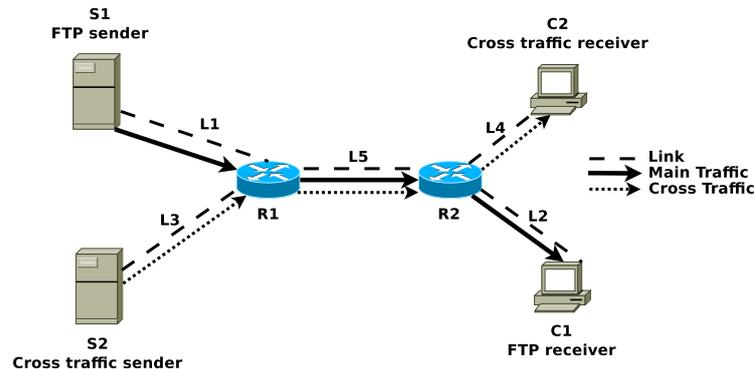
Figure 4.1: Emulated network using Mininet
