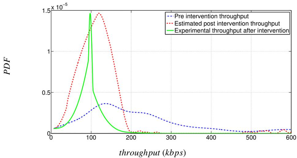
Figure 4.3: Effect of an intervention on the retransmission score, on the throughput distribution
