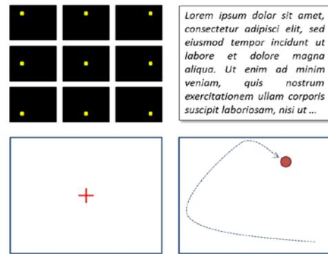
**Figure 1. Eye movement stimuli:** top-left, jumping-point; top-right, text; bottom-left, static cross; bottom-right, moving object.
