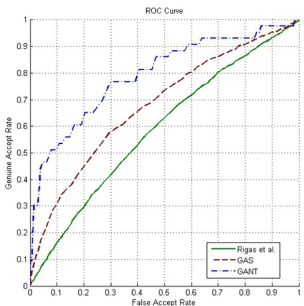
**Figure 5. CMS and ROC curves for experiment 1. Results for all three methods when using Round 2 as Gallery set and Round 1 as Probe set.** Score curve (CMS) and Receiver Operating Characteristic curve (ROC) curves indicating Rigas et al. performances on our database are presented.
