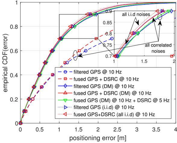
Fig. 10. Positioning performance comparison of different schemes assuming correlated GPS noise and correlated shadowing except the two dotted curves of the all i.i.d. cases in the urban canyon scenario.
