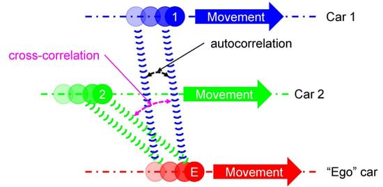
Fig. 2. Possible shadowing autocorrelations/cross-correlations on/between V2V link(s) having dual mobility in VANETs.
