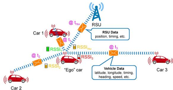
Fig. 1. Cooperative cars periodically exchange CAM messages to maintain awareness of each other and to support distributed CP. Both the transmission time  $@t_i$  and the received power level  $RSSI_i$  depend on the transmission car  $i$  (and thus, on the V2V link).
