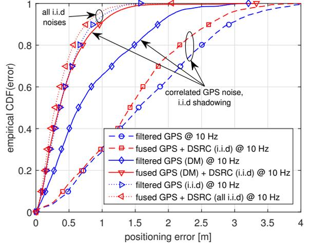
Fig. 7. Positioning performance comparison of different schemes assuming correlated GPS noise and i.i.d shadowing except the two top curves of the all i.i.d cases in the highway scenario.
