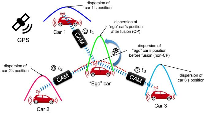
Fig. 3. “Ego” car receiving asynchronous CAMs from 1-Hop “virtual anchors” to perform distributed CP. The dispersion of CP location estimates (i.e. through GPS+DSRC) is expected to be lower than that of non-CP estimates (i.e., standalone GPS).
