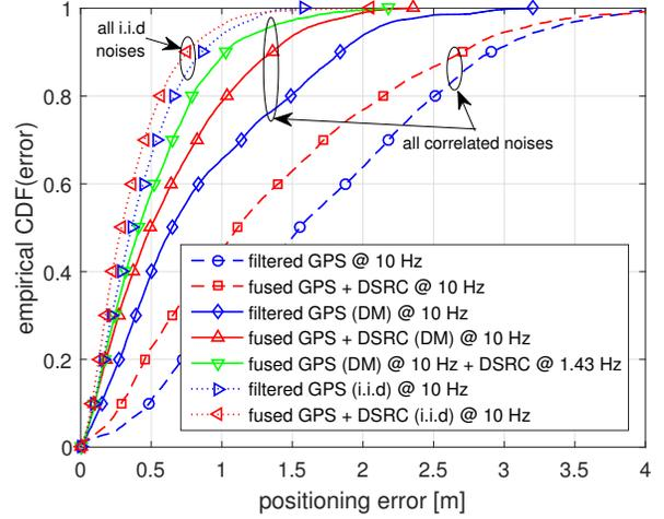
Fig. 9. Positioning comparison of different schemes assuming correlated GPS noise and correlated shadowing except the two top curves of the all i.i.d cases in the highway scenario.
