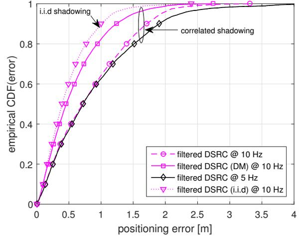
Fig. 11. Positioning performance comparison of different schemes assuming loss of GPS signal and correlated shadowing except the top curve of i.i.d. shadowing in the tunnel scenario.
