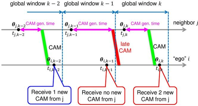
Fig. 5. Impacts of asynchronous position estimates and CAM transmissions on the information fusion.
