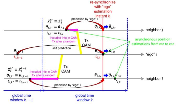
Fig. 4. Example of the space-time schematic managed by the “ego”  $i$  whose neighbors are vehicle  $j$  and  $l$ . Due to asynchronous estimates, the “ego”  $i$  needs to perform prediction of received information at its time of interest  $t_{i,k}$ .
