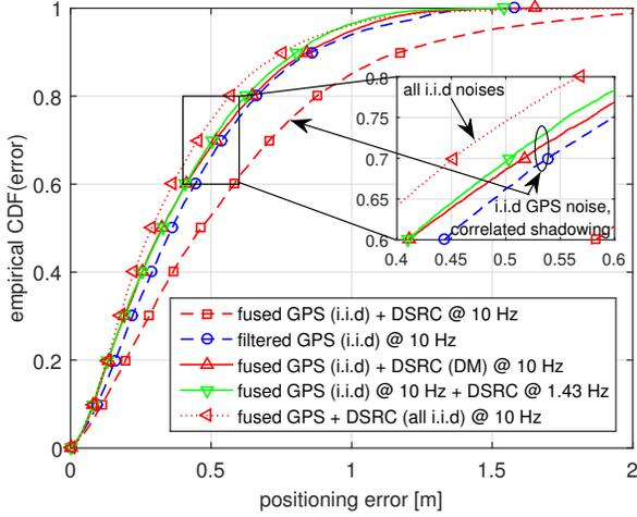
Fig. 8. Positioning performance comparison of different schemes assuming i.i.d GPS noise and correlated shadowing except the top curve of the all i.i.d case in the highway scenario.
