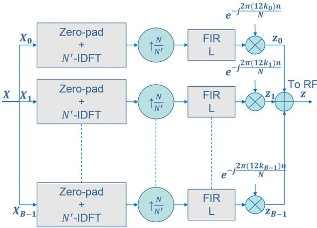
Fig. 3. Architecture of improved UFMC transmitter
