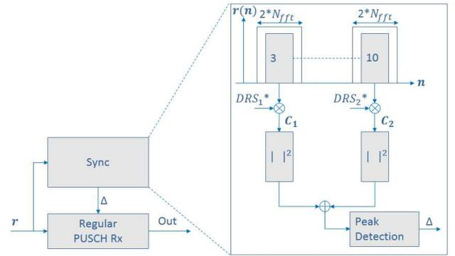
Fig. 5. Structure of proposed UFMC receiver
