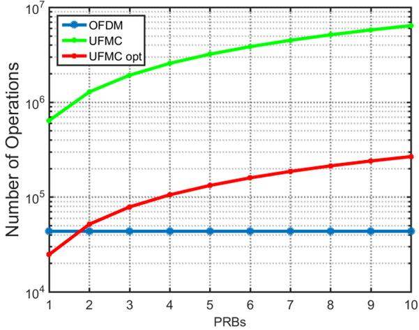
Fig. 6. Complexity of OFDM(blue), classical(green) and proposed(red) UPMC modulators
