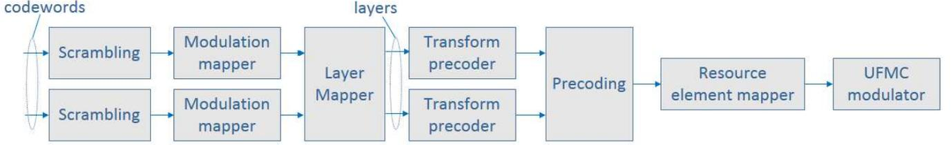
Fig. 1. Architecture of the UFMC transmitter
