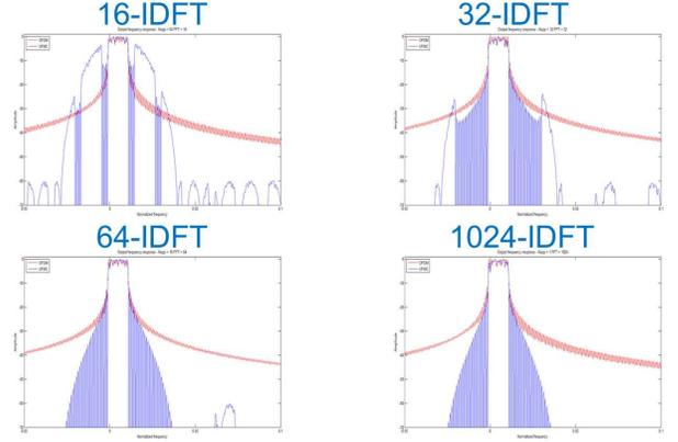
Fig. 4. UFMC spectrum(blue) and OFDM spectrum(red) versus IDFT size
