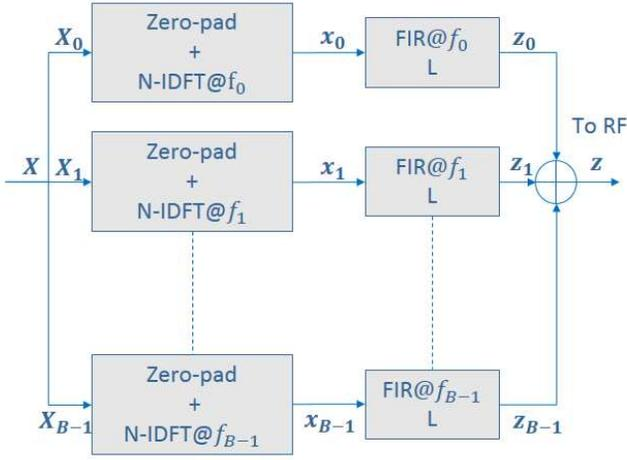
Fig. 2. Architecture of classical UFMC transmitter
