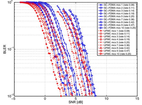
Fig. 7. Performance evaluation (BLER vs SNR) of the UPMC receiver in an AWGN channel.
