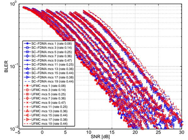
Fig. 8. Performance evaluation (BLER vs SNR) of the UPMC receiver in a Rayleigh fading channel
