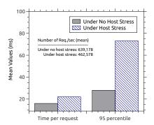
Fig. 2: Stressing Apache service at a host machine.
