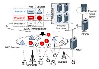
Fig. 1: The MEC concept in LTE networks and services offering by multiple different tenants (service providers).
