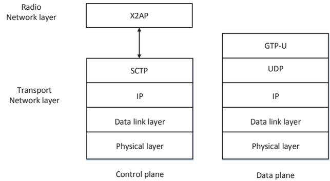
Fig. 1. eNB X2 protocol stack for control-plane and data-plane
