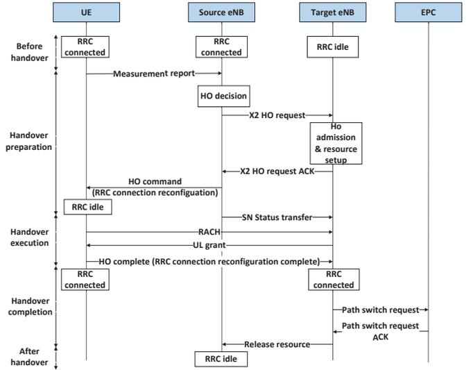
Fig. 2. X2 handover procedure
