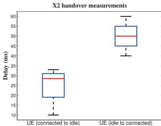
Fig. 4. X2 handover measurements
