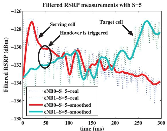
Fig. 6. RSRP measurements both for source eNB (serving cell) and target eNB (target cell) for  $S=5$
