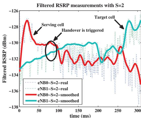
Fig. 5. RSRP measurements both for source eNB (serving cell) and target eNB (target cell) for  $S=2$
