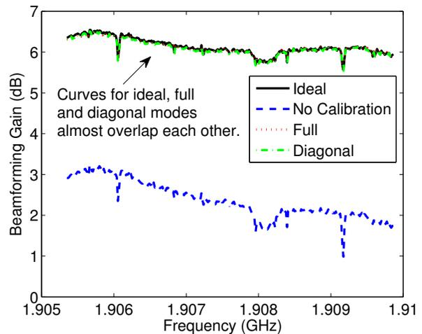
Fig. 4: Beamforming gain of a  $4 \times 1$  MISO system with regard to a SISO system under the assumption of ideal calibration, no calibration, calibration assuming a diagonal matrix and calibration assuming a full matrix (SNR averaged over 28 random locations) [12].
