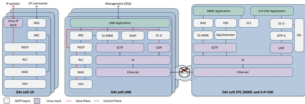
Fig. 1: OpenAirInterface LTE software stack.
