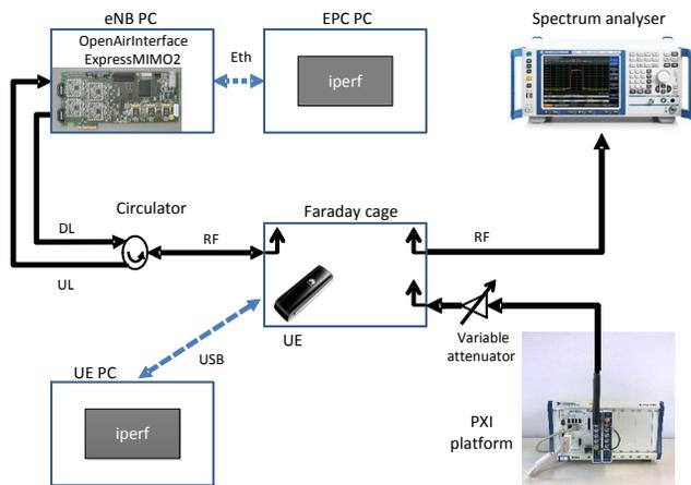
Fig. 5: Experimental setup for 4G/5G co-existence testing [13].
