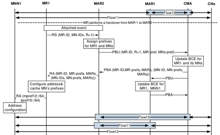
Fig. 4: Signaling flow for MR handover between two MARs.
