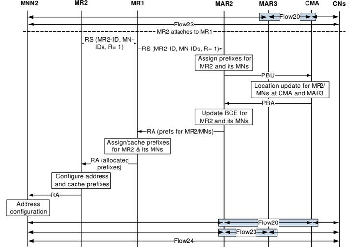
Fig. 6: Signaling flow for a Nested NEMO scenario.
