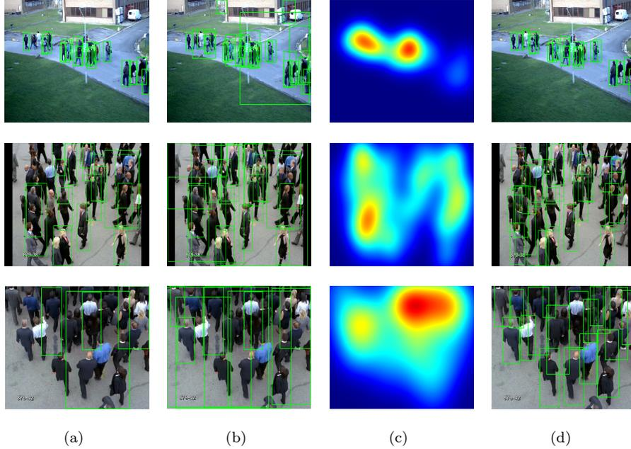
Figure 4: Exemplary visual results comparing the performance of crowd-sensitive threshold to the baseline method: (a) baseline algorithm at  $\tau_{max}$ , (b) baseline algorithm at  $\tau_{min}$ , (c) estimated crowd density map, (d) proposed method using dynamically chosen  $\tau_{dyn}$  computed from the density values and correction filter according to aspect ratio and perceived height. From top to bottom: Frames from PETS, UCF 879, and INRIA 879-38.
