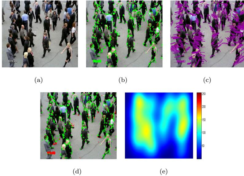
Figure 2: Illustration of the proposed crowd density map estimation using local features tracking: (a) exemplary frame, (b) FAST local features (c) feature tracks (d) distinction between moving (green) and static (red) features - red features at the lower left corner are due to text overlay in the video (e) estimated crowd density map.
