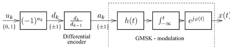
Fig. 2. Signal flow diagram for the GMSK modulation.
