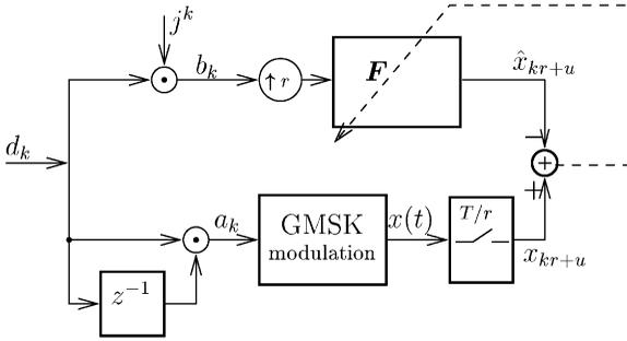
Fig. 3. Identification of the GMSK modulation by least squares.
