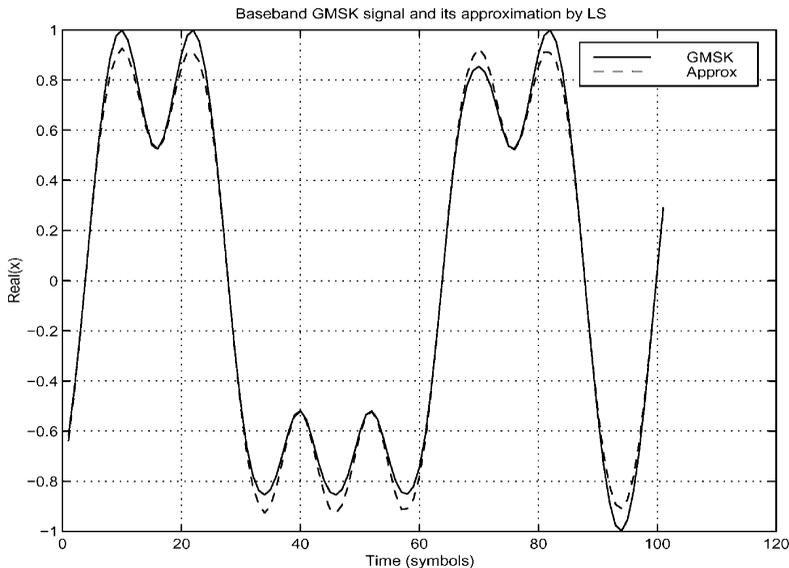
Fig. 4. Linearization of a baseband GMSK signal.
