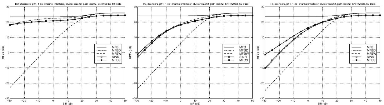
Fig. 6. MFB vs. SIR for SNR = 20 dB, two sensors, one interferer and no oversampling, for RU, TU and HI channel models.
