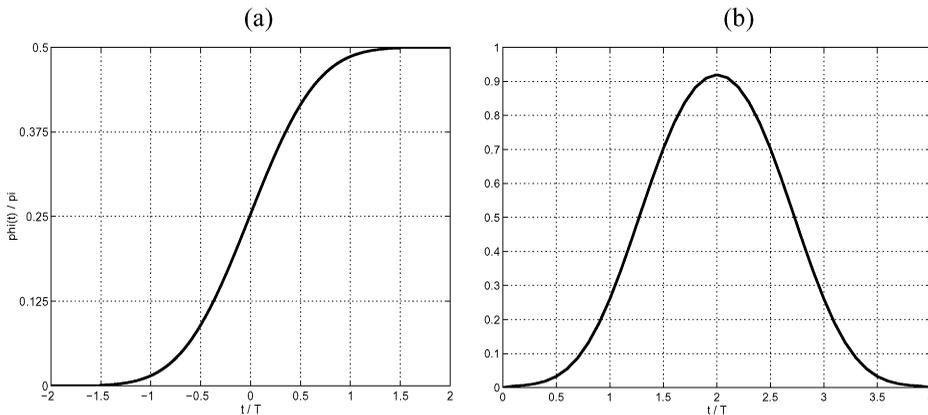
Fig. 1. (a) Phase impulse response  $\phi(t)$  of the GMSK modulation, (b) GMSK pulse shape filter  $f(t)$ .
