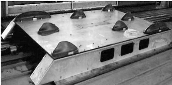
Fig. 6. Antennas on top of the IRIS 320 train.
