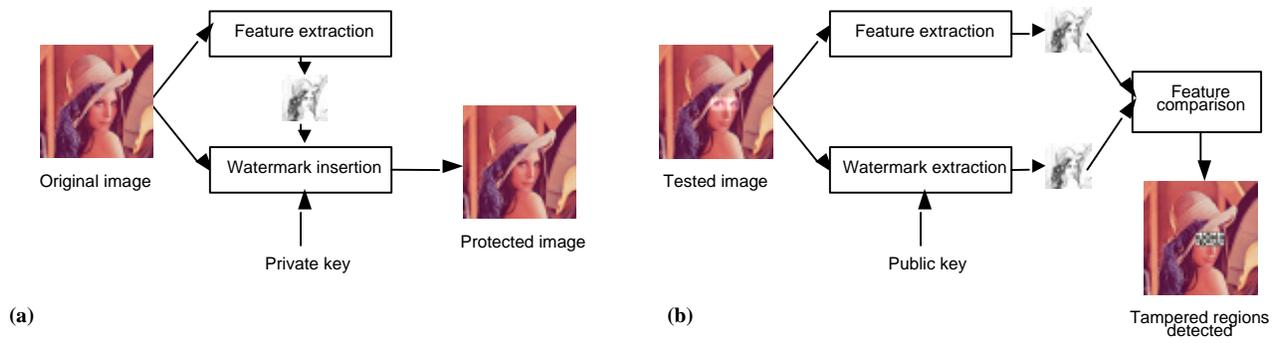
Figure 3 – Generic robust watermark scheme: (a) Image security, (b) Authenticity verification
