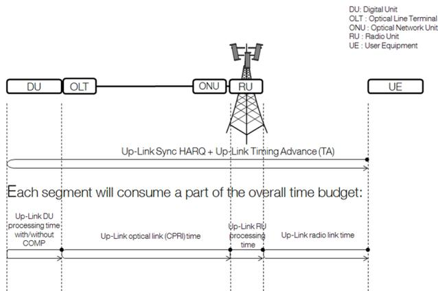
Fig. 7. Network and equipment segments to be considered for fronthaul latency.
