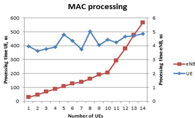
Fig. 5. MAC layer profiling - uplink & downlink
