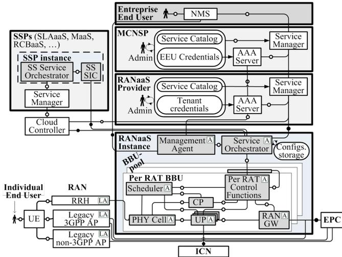
Fig. 2. MCN RANaaS architecture (extracted from [5]).
