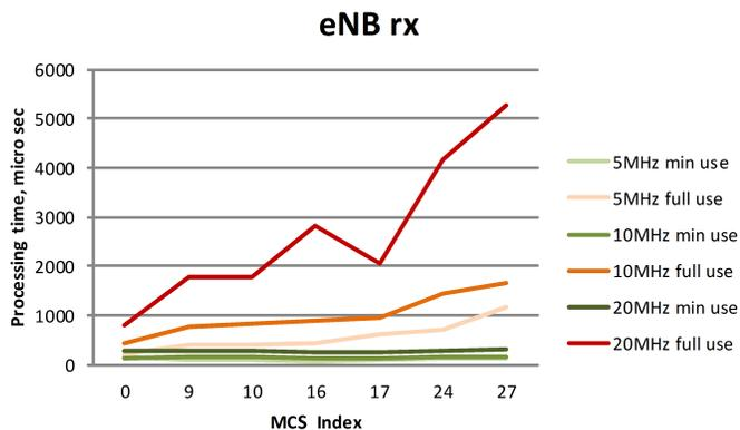
Fig. 4. PHY layer profiling - uplink
