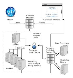
Figure 1: Architecture of the entire system.
