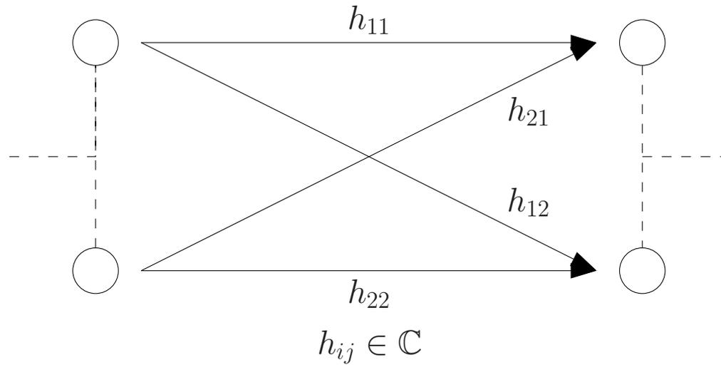
Multiple antenna transmission between cooperating antenna arrays
