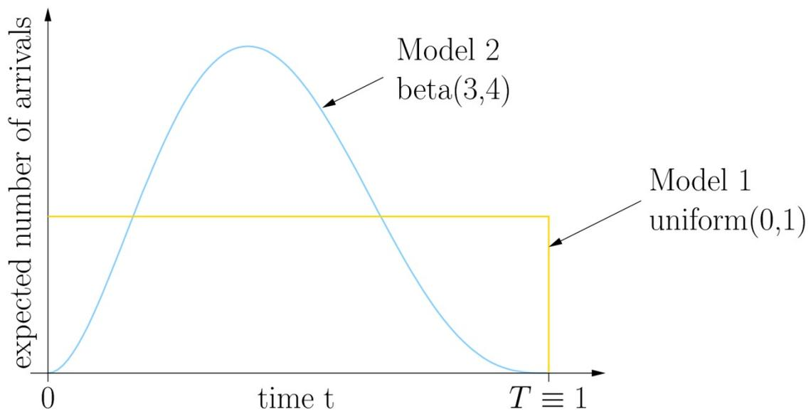
Figure 5: Access intensity of the 3GPP model.
