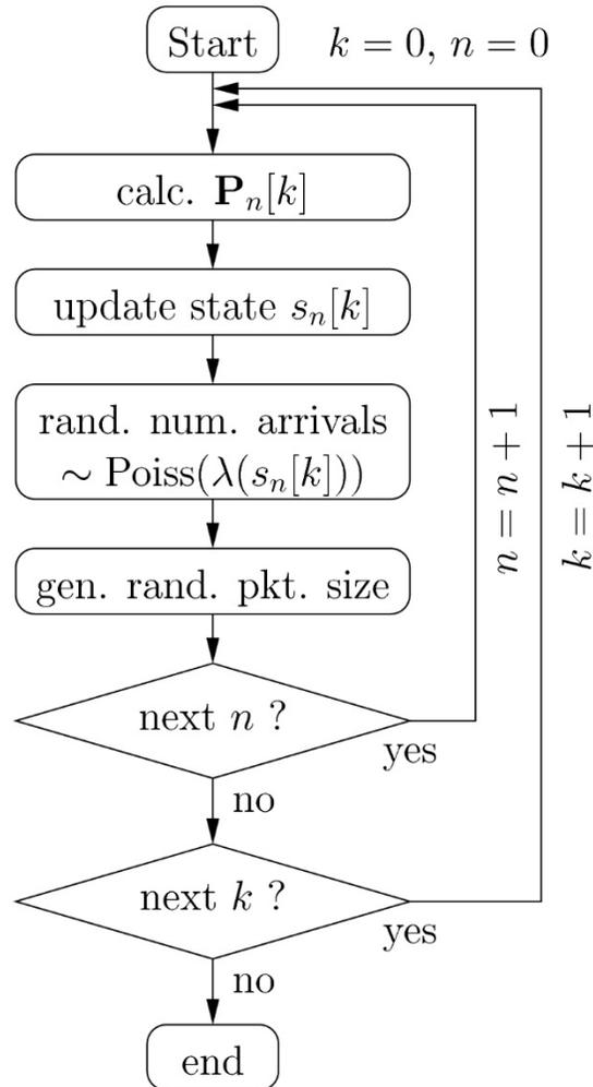
Figure 9: Generation of samples from the CMMPP model; the indices  $n$  and  $k$  stand for the device and time instant, respectively.
