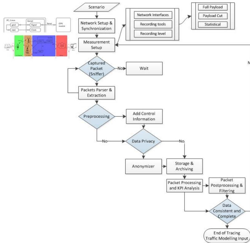
Figure 2: Packet tracing workflow.
