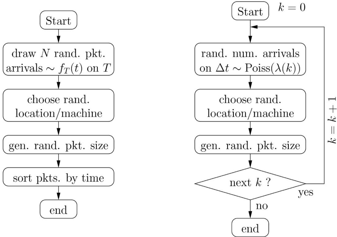
Figure 7: Generation of samples from the 3GPP model. Left: non-sequential, right: sequential.
