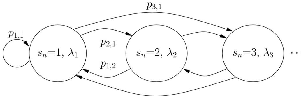
Figure 8: Markov chain driving the MMPP model.
