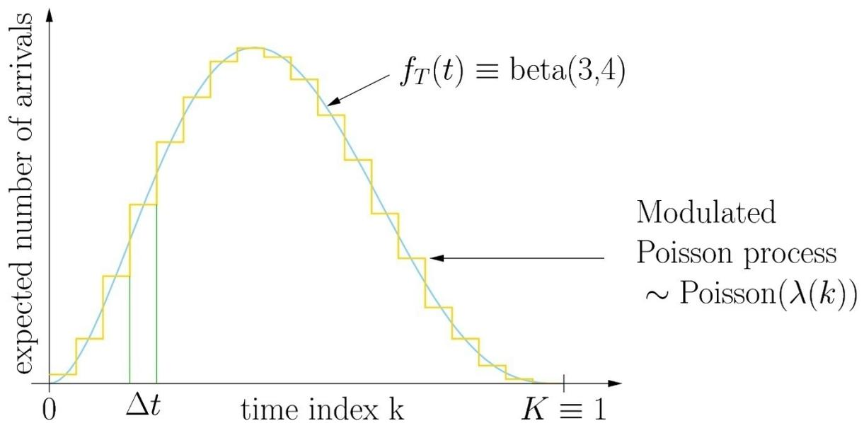
Figure 6: Synthesis of the 3GPP model from a modulated Poisson process.
