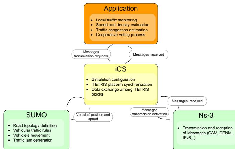
Figure 2 The iTETRIS simulation system, where iCS stands for iTETRIS Control System.
