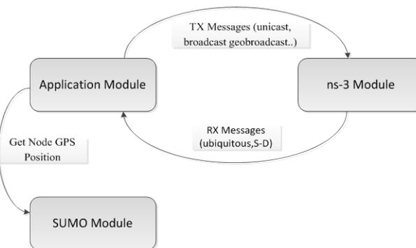
Figure 4 Application module interaction with ns-3 and SUMO through subscriptions
