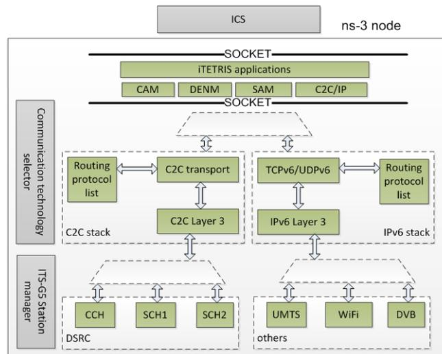
Figure 3 ns-3 V2X stack architecture and components, where C2C stands for Car-2-Car, and CCH, SCH, stands for Control Channel and Service Channel, respectively.
