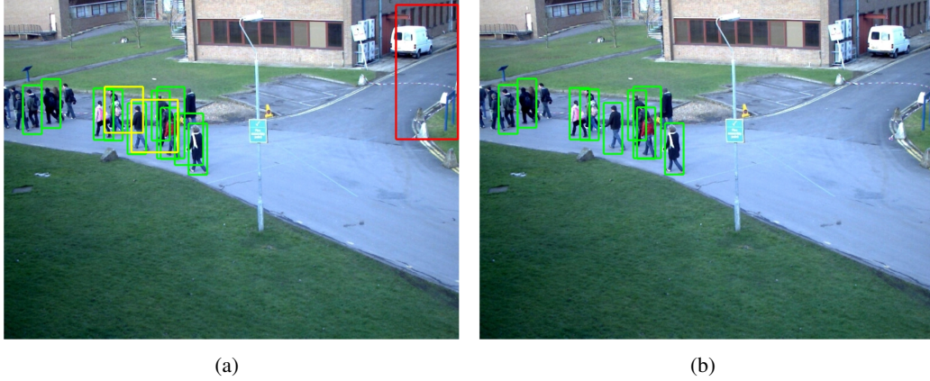
Figure 6.2: Exemplary effects of the proposed correction filters on a frame from PETS 2009 dataset [41]: (a) detections without filtering, (b) filtering according to aspect ratio and perceived height. While the unfiltered detections might include too large candidates (red) and also detections comprising several persons at correct height (yellow), the aspect ratio and perceived height allow removing most of them.
