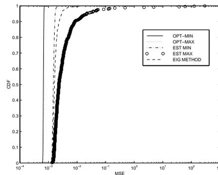
Figure 4: User 1 MSE cumulative distribution function for single user Bayesian channel estimation (SNR = 20dB for user 1, SNR=30dB for interferers).
