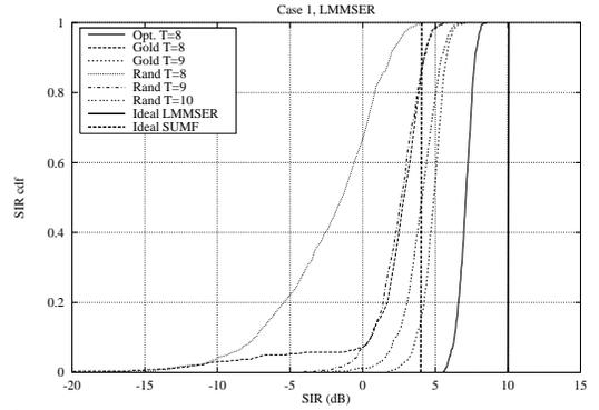
Figure 1: User 1 SIR cumulative distribution function for the MMSE receiver with joint channel estimation (SNR = 15dB for all users).
