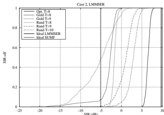
Figure 2: User 1 SIR cumulative distribution function for the MMSE receiver with joint channel estimation (SNR = 15dB for users 1 and 2, other users SNR = 25 dB).
