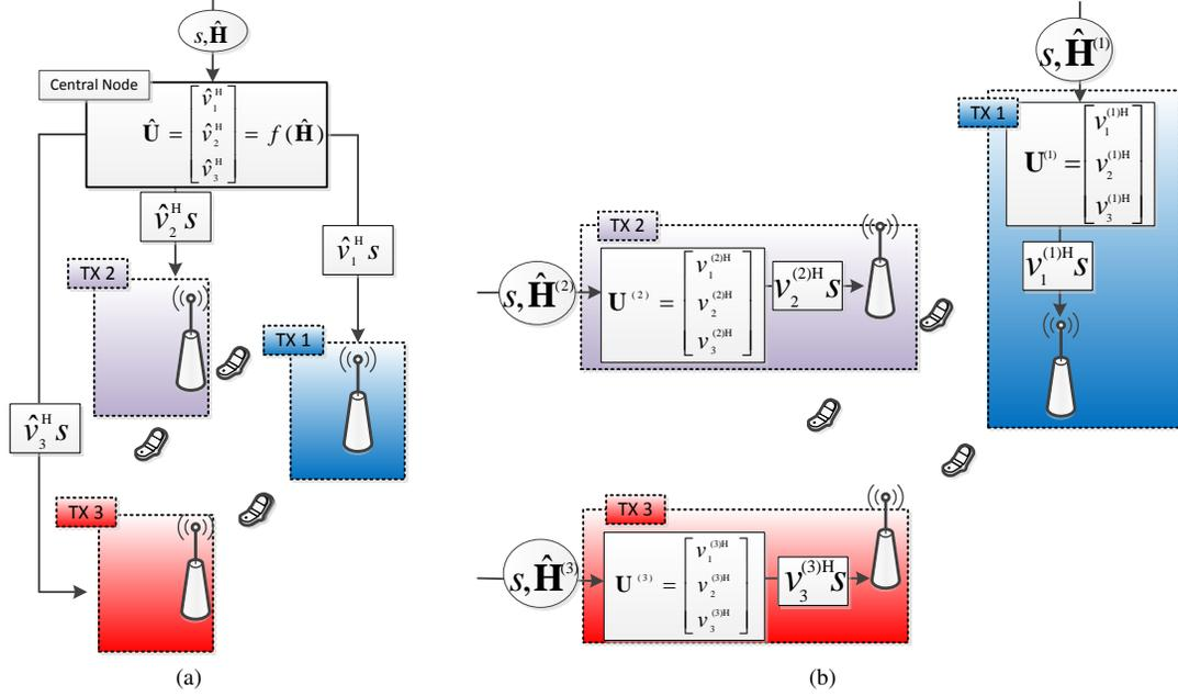
Fig. 1: The transmission with centralized CSIT/precoding is symbolically represented in Figure (a) while Figure (b) represents the distributed CSIT/precoding .
