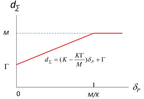
Fig. 4. Achievable sum DoF  $d_\Sigma$  vs.  $\delta_P$  for the MISO BC with  $M < K$ .
