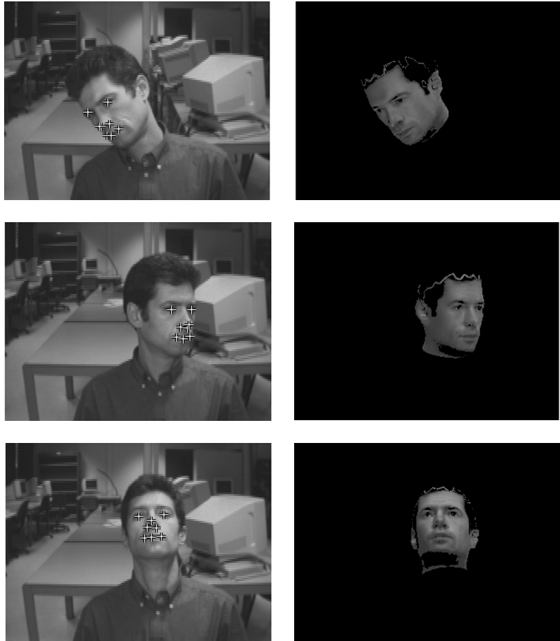
Figure 2. Head rotations supported by the face tracking system, without any marker or specific lighting.
