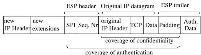
Fig. 8. Structure of IP datagrams in tunnel mode ESP
