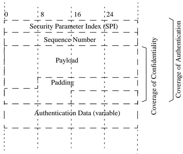
Fig. 6. Main fields of the ESP Header
