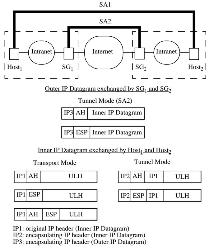
Fig. 11. Combined VPN and end-to-end security with IPsec
