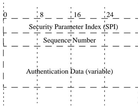
Fig. 2. Main fields of the IP Authentication Header
