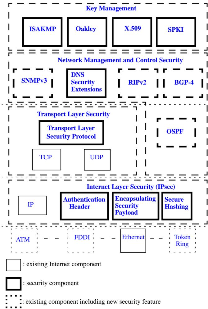
Fig. 1. Cryptographic security components of the Internet infrastructure
