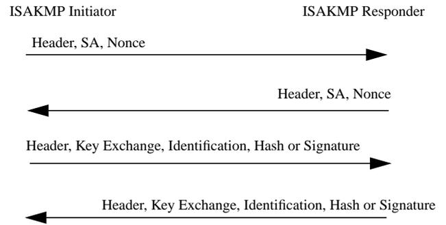
Fig. 16. Message flow for the base ISAKMP exchange
