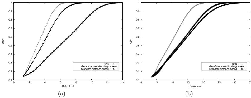
Fig. 14: The CDF of the average information reception delay in case of BZB, flooding and standard distance-based approaches. (a) Packet size 500 bytes. (b) Packet size 2200 bytes.
