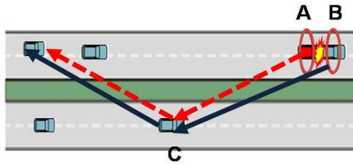
Fig. 21: An illustration of a scenario where two nodes detect the same emergency event and send different packets to the network.
