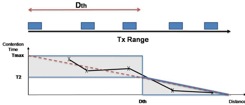
Fig. 7: The BZB contention scheme where the dashed and the plane curves represent respectively the distance-based CBF waiting time and the bounds of BZB.
