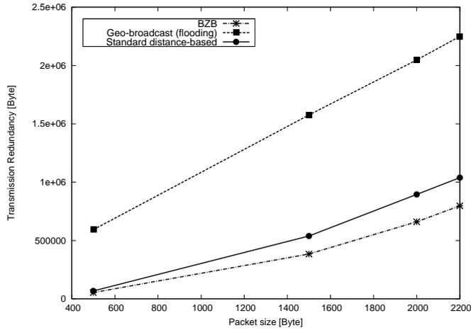
Fig. 11: The variation of the transmission redundancy factor in case of BZB, flooding and standard distance-based approaches with regards to the payload.
