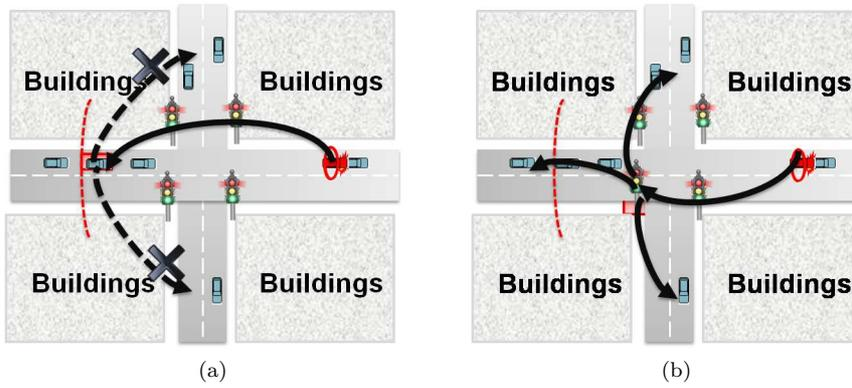
Fig. 6: Road Side Unit role in the dissemination process. (a) The first case where the vehicle is selected as the next relay. (b) The second case where the RSU is selected as the next relay.
