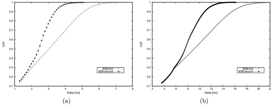
Fig. 15: The CDF of the average information reception delay. (a) Packet size 500 bytes. (b) Packet size 2200 bytes.
