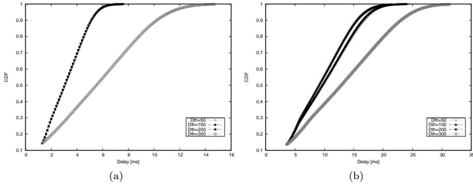
Fig. 20: The CDF of BZB delay when varying the  $D_{th}$  value. (a) Packet size 500 bytes. (b) Packet size 2200 bytes.
