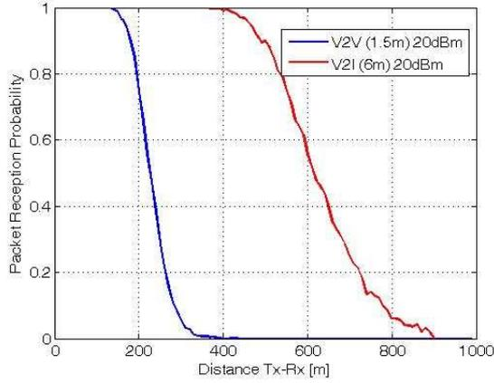
Fig. 5: A representation of the capabilities of V2V communications (with an antenna height of  $1.5m$ ) vs. V2I communications (with an antenna height of  $6m$ ) [2].
