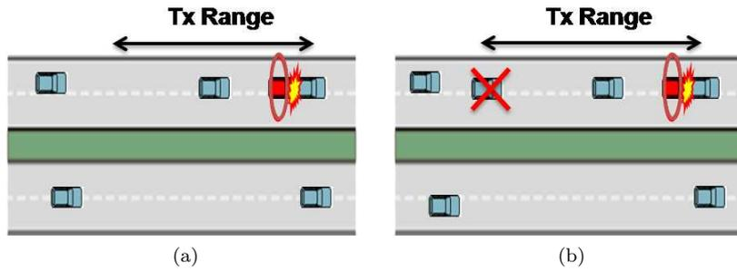
Fig. 3: First limitation of the distance-based dissemination approach. (a) There are no distant nodes at the border of the radio range of the transmitter due to the non uniform distribution of vehicles. (b) Farthest nodes from the transmitter can not receive correctly the message due to fading phenomena.
