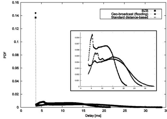
Fig. 13: The PDF of the average information reception delay in case of BZB, flooding and standard distance-based approaches for packet size 2200 bytes.
