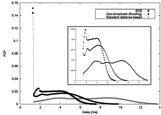
Fig. 12: The PDF of the average information reception delay in case of BZB, flooding and standard distance-based approaches for packet size 500 bytes.
