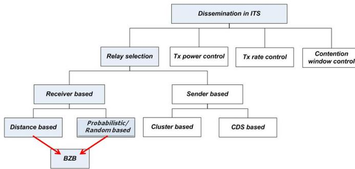
Fig. 1: Classification of dissemination approaches proposed for ITS systems.
