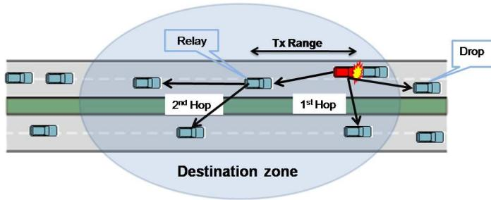
Fig. 2: Illustration of an example of a road situation where a vehicle in a dangerous situation issues emergency messages. The distance-based CBF is used to propagate the information in the destination zone. The farthest node in the communication range is always selected to relay the message. Nodes outside the destination zone are not involved in the dissemination process.
