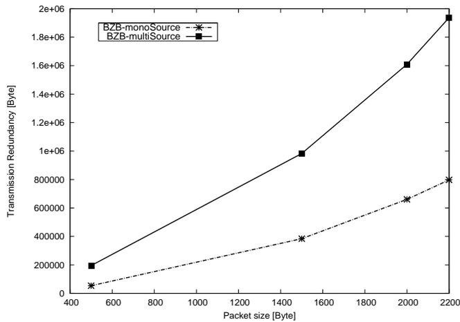
Fig. 22: The variation of BZB transmission redundancy factor with regards the payload in case of multiple sources scenario.
