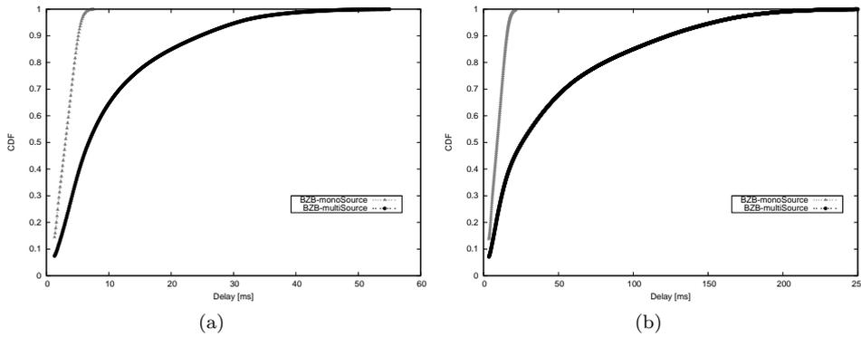
Fig. 23: The CDF of BZB delay in multiple sources scenario. (a) Packet size 500 bytes. (b) Packet size 2200 bytes.
