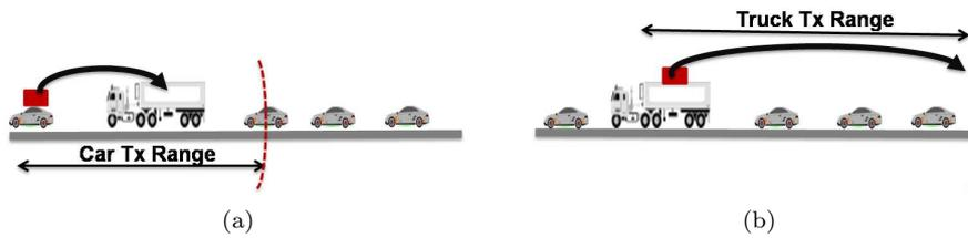
Fig. 4: Impact of the participation of the vehicles with important antenna height in the dissemination process. (a) The first case where the farthest car can not act as the next relay because the signal is hidden by the truck. (b) The second case where the truck is selected as the next relay.
