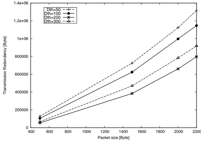
Fig. 19: The BZB transmission redundancy factor when varying the  $D_{th}$  value with regards the payload
