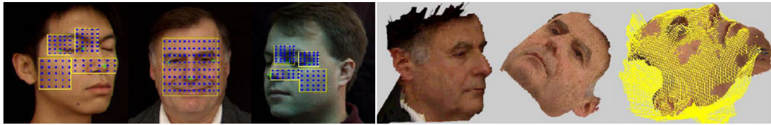
Figure 7: (Left) Control point ( \sim 100 ) selection for a left profile, frontal and right profile scan (Right) Matching result after fine alignment of the 2.5D test scan (wireframe) to the 3D model (textured) (Lu, et al., 2004).
